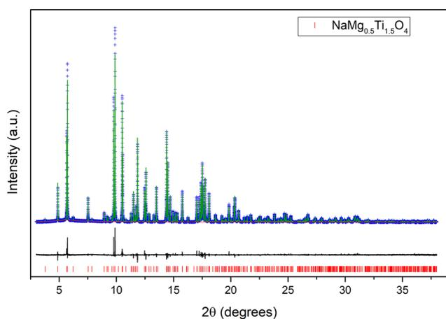
**Figure 3.** Rietveld refinement using synchrotron data for  $\text{NaMg}_{0.5}\text{Ti}_{1.5}\text{O}_4$ . Blue crosses are the observed intensities, the green curve is the fitted pattern, the black curve is the difference pattern, and the red tick marks indicate the location of the CF- $\text{NaMg}_{0.5}\text{Ti}_{1.5}\text{O}_4$  peaks.
