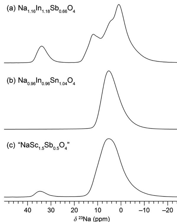
**Figure 6.**  $^{23}\text{Na}$  solid-state NMR spectra at 12.5 kHz MAS and 9.4 T: (a)  $\text{Na}_{1.16}\text{In}_{1.18}\text{Sb}_{0.66}\text{O}_4$ , (b)  $\text{Na}_{0.96}\text{In}_{0.96}\text{Sn}_{1.04}\text{O}_4$ , and (c) “ $\text{NaSc}_{1.5}\text{Sb}_{0.5}\text{O}_4$ ” central transition resonances.
