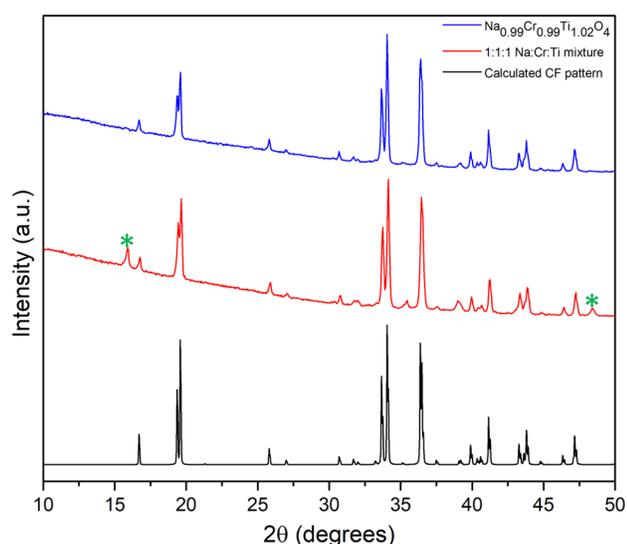
**Figure 4.** Powder XRD patterns for the 1:1:1 and 0.99:0.99:1.01 Na/Cr/Ti samples compared to a calculated pattern for the CF phase. Asterisks highlight peaks from the secondary phase  $\text{Na}_{0.6}\text{Cr}_{0.6}\text{Ti}_{0.4}\text{O}_2$  in the 1:1:1 Na/Cr/Ti sample.
