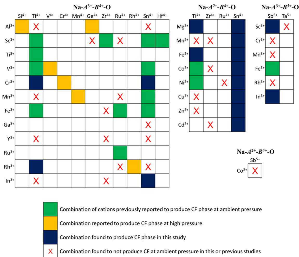
**Figure 5.** A combinatorial representation of the Na-CF phase space. The phase-space shown covers all Na-CF compounds and combinations known to have been attempted in previous studies or this work. Conceivable but unexplored combinations (e.g.,  $\text{Sc}^{3+}$  and  $\text{Mo}^{4+}$ ) are not depicted.
