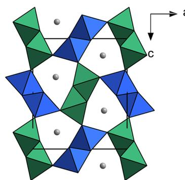
**Figure 1.**  $\text{CaFe}_2\text{O}_4$  structure. Gray spheres represent  $\text{Na}^+$ . Green and blue octahedra represent the two symmetrically independent framework sites comprising the two “double rutile” chains.
