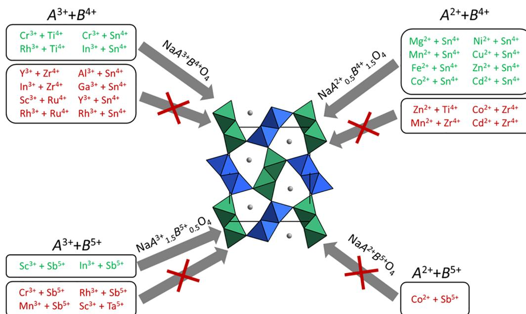
**Figure 2.** Schematic summarizing the synthetic approach and results presented in this paper. The ion combinations in green were successfully synthesized in the postspinel structure, whereas the ion combinations in red formed alternative phases.
