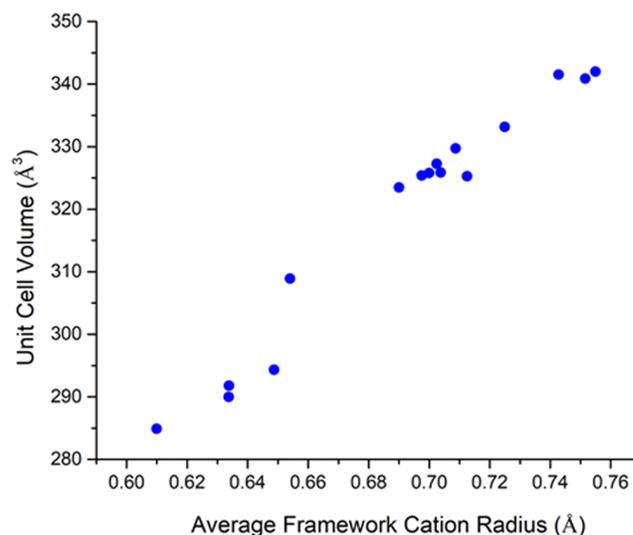
**Figure 7.** Unit cell volume of the new Na-CFs versus the weighted-average effective ionic radius of the framework cations in octahedral coordination.<sup>58</sup>
